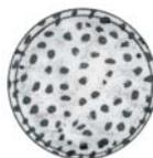
Cavities are beginning to form. Grinding necessary.
