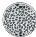
Limits of erosion exceeded. New tip necessary.
