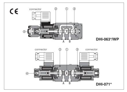
Spool type, two or three position, direct operated valves with solenoids certified according the North American standard **cURus**.
