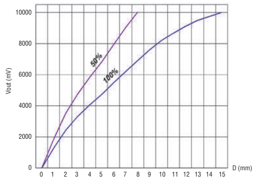
K50G30V010 al 50% e al 100% della portata K50G30V010 at 50% and at 100% sensing distance 24 VDC @ 20°C @ RLOAD = ∞
