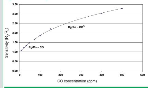
Sensitivity over range 8 -500ppm CO operating in 2temperature mode with a 5:1 cycle ratio of sensing (400°C) and resetting (525°C). Note linear behaviour <50ppm and power law behaviour >50ppm.
