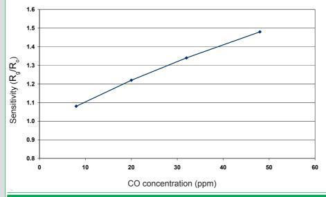
Sensitivity over range 8-50ppm CO operating in 2temperature mode with a 5:1 cycle ratio of sensing (400°C) and resetting (525°C). Linear behaviour is observed.
