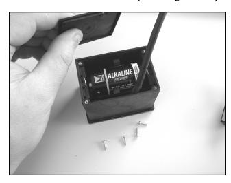
Now the commercial baby cell (1,5 V/8 Ah) can be changed. All datas (except the actual position) will be stored in the data memory.
