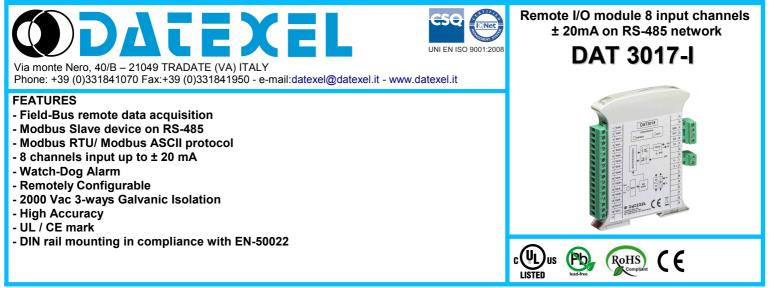
GENERAL DESCRIPTION The device DAT 3017-I is able to acquire up to 8 analogue input signals. The data are transmitted with MODBUS RTU/MODBUS ASCII protocol on the RS-485 network (RS-232 interface is available).
