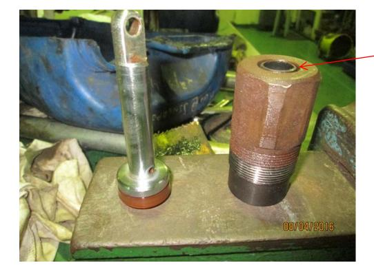
Seal as well as O-rings Required(Oil leaking from this area)
