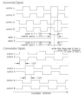
NOTE: ALL DEGREE REFERENCES ARE ELECTRICAL DEGREES. WAVEFORM SHOWN WITH OPTIONAL COMPLEMENTARY SIGNALS  $\overline{A}, \overline{B}, \overline{Z}$  FOR HV AND OD OUTPUTS ONLY.
