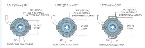
\*Order Appropriate No Charge Mounting and Installation Kit for SB, SC, or SD Option. Each kit contains 10 screws for mounting 5 encoders.
