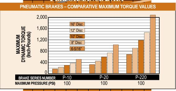
These graphs have been included for quick reference. Intended for use as a general guide, they reflect the maximum torque values possible with each brake and disc combination.
