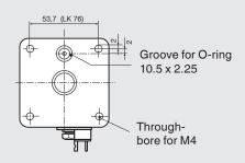
Dimensions [mm] GW...A4/2 HP IP 65 with metal housing, cable entry M 20 x 1.5
