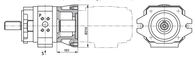
PGH5 with combination part for PGH4, A10VO45 (SAE-B flange, shaft 15T 16/32 DP)
