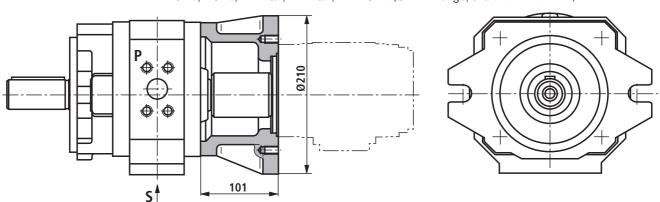
PGH5 with combination part for PGH2, PGH3, PGF2, PGP2, G2-4X, A10VSO10/18 (SAE-A flange, shaft 9T 16/32 DP)
