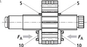
Axial longitudinal gaps between rotating and fixed parts are therefore extremely small, which ensures optimum axial sealing of the pressure chamber.
