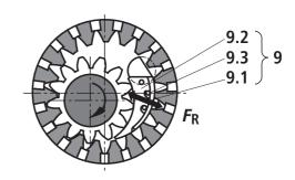
Depending on the operating pressure, the two segment elements (9.1) and (9.2) are pressed against the crowns of the teeth on pinion shaft (3) and hollow gear (2).
