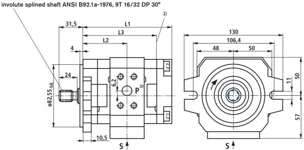
S = Standard pressure series; for precise dimensions, see table on page 17 (2) For multiple pumps the combination part starts here
