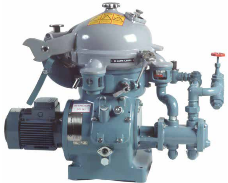
Fig 1. MAB 104B-14/24, with feed and discharge pump.
