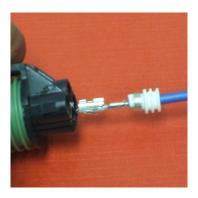
Photograph CK1I05, showing the crimp pin insertion orientation
