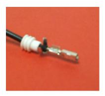
Photograph CK1I02, showing some partly crimped flaps
