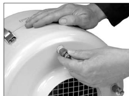
**(GB)** Fit foam collar seal around inlet spigot supplied` with unit).
