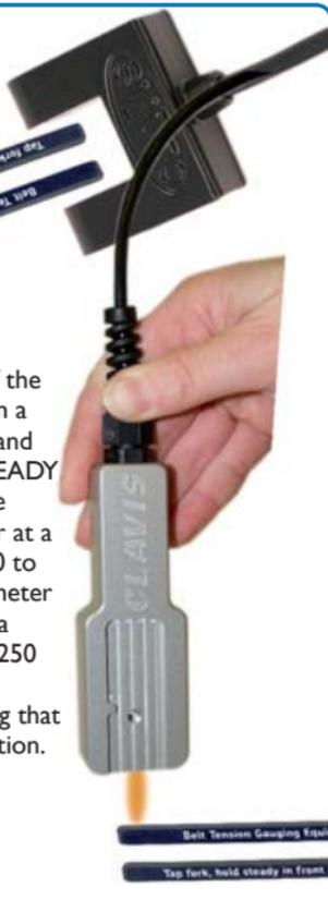
Results within  $\pm 1\%$  are acceptable. There is no adjustment possible. If greater variance is experienced, the meter should be returned for calibration. See section 7.2 for manufacturer's contact information.
