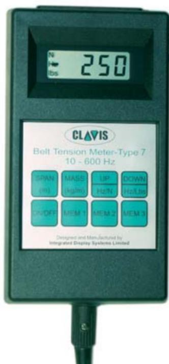
Tap the tip of the tuning fork on a hard surface and then hold STEADY in front of the optical sensor at a distance of 10 to 15 mm. The meter will measure a frequency of 250 Hz thus demonstrating that it is in calibration.
