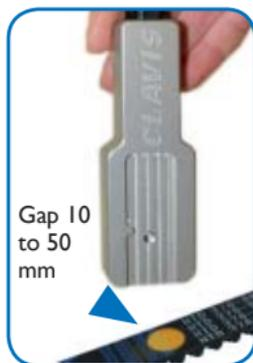
Place sensor across the selected belt span at the mid-span position. Make sure that the jaws of the sensor do not touch the belt.
