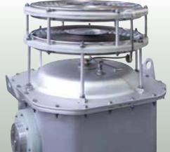
Detail of a rupture disc in a CG head.
