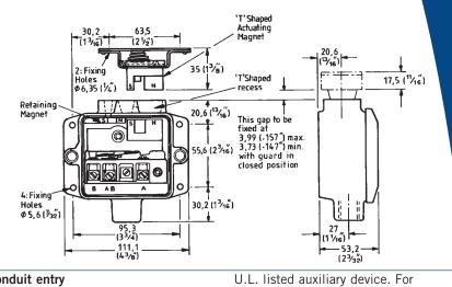
**Conduit entry** Model 30800: M20 x 1.5 to B.S. 4568 Model U30800: <sup>1</sup>/<sub>2</sub>" - 14 NPT Model C30800: <sup>1</sup>/<sub>2</sub>" - 14 NPT
