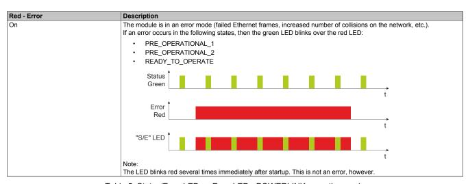
Table 5: Status/Error LED as Error LED - POWERLINK operating mode
