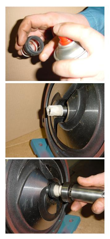
1) Lubricate the O-ring and the sealing surfaces with oil.
