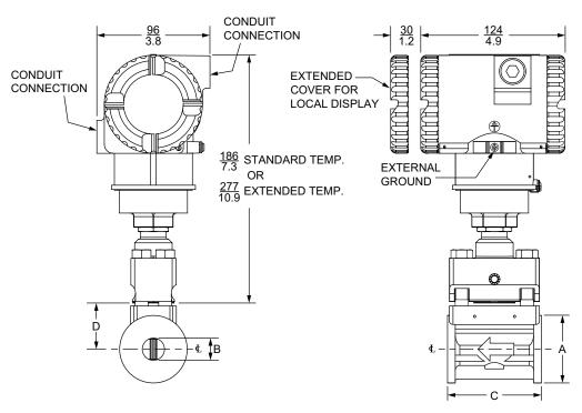
Figure 7 - Wafer Body Flowmeter with Junction Box
