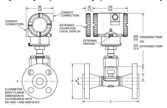
Figure 4 - Flanged Body Flowmeter with Junction Box
