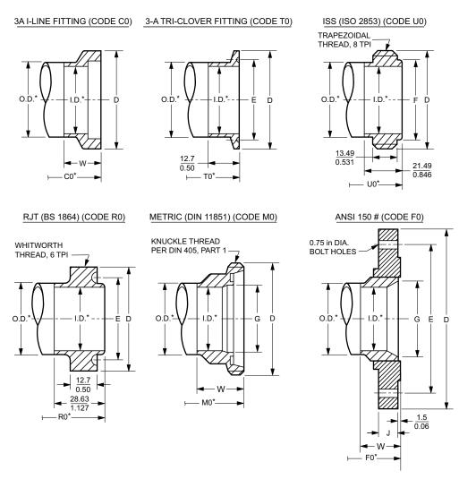
**NOTE:** Refer to Sanitary Flowmeter Body Dimensions, page 60 for values of O.D., I.D., and tube lengths C0, T0, U0, R0, M0, and F0.
