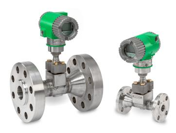
When configured with Multivariable selection T, the Model 84C Vortex flowmeter provides a process temperature measurement using the optional integral temperature sensor. With calculations based on ASME steam tables<sup>3</sup>, the Model 84C is an excellent solution for the mass flow metering of saturated steam.
