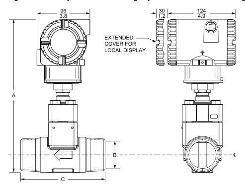
Figure 10 - NPT Body Flowmeter with Junction Box
