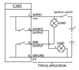
NOTE: IF SINK ONLY OUTPUT IS REQUIRED THEN PIN A IS NOT USED.
