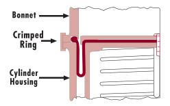
Fig. 29: Crimped Ring
