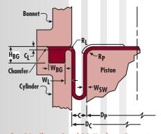
Fig. 24: Classes 3 and 3C Hardware Dimensions
