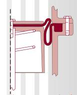
Fig. 18: Diaphragm inversion resulting from lack of curved retainer plate.
