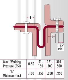
Fig. 36: Hole Spacing Dimensions
