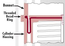
Fig. 31: Bezel Ring or Grooved Bonnet
