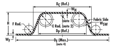
Diaphragms are shown in the "as molded" configurations. The diaphragm must be inverted prior to installation.
