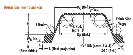
Diaphragms are shown in the "as molded" configuration.
