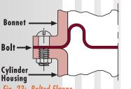
Fig. 23: Bolted Flange
