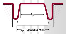
Fig. 40: Tapering the Piston
