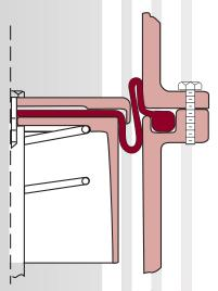
Fig. 38: Pressure Reversal of Diaphragm
