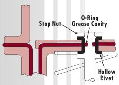
Fig. 39: Slip Joint Shaft Assembly
