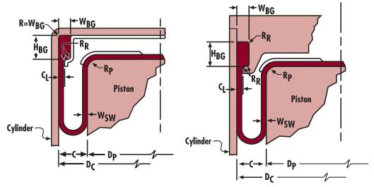
Fig. 32: Axial Compression with Stamped Retainer Plate
