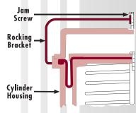
Fig. 26: Pivot Rocking Bracket
